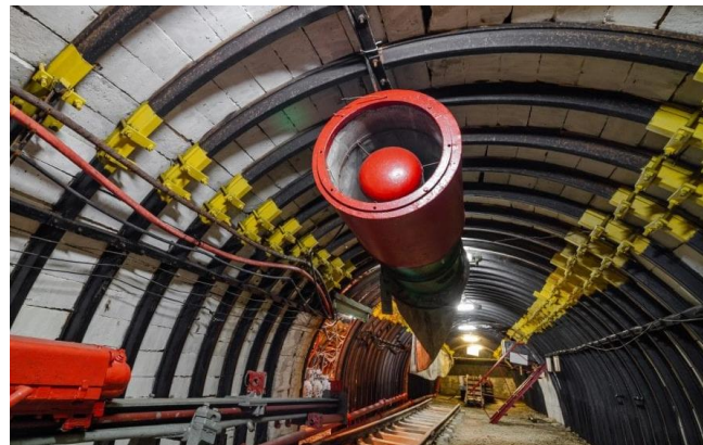
Figure 8. Effective mine ventilation provides fresh air to miners and abatement of dust, mine gases, and exhaust fumes that accumulate in the work area.
