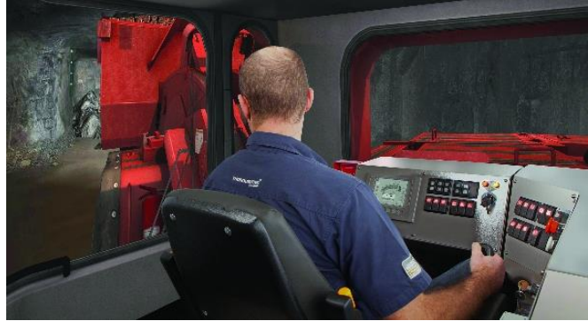
Figure 6. Diesel exhaust and dust protection is afforded by properly enclosed cabs on underground mine machinery.
