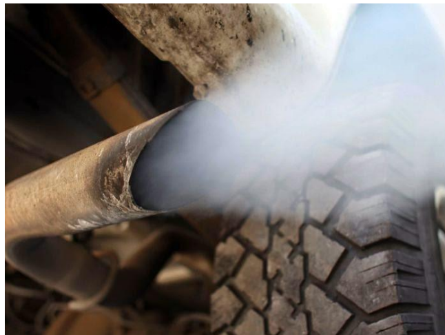
Figure 4. The exhaust from diesel engines contains a mixture of gases and very small particles that can create a health hazard when not properly controlled.
