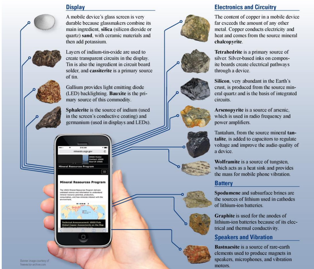
Figure 1. Cell phone and the minerals used for components in mobile devices. (Source United States Geological Survey)
