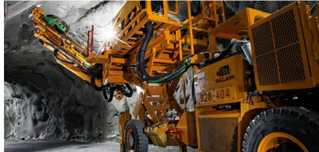
Figure 3. Battery electric powered mining equipment is gaining acceptance in underground mining operations.
