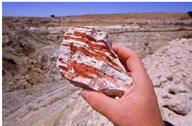
Figure 1. Bentonite is a naturally occurring rock that is composed predominantly of the clay mineral smectite. Most bentonites are formed by the alteration of volcanic ash in marine environments and occur as layers sandwiched between other types of rocks.
