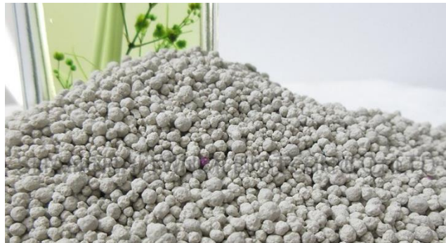
Figure 2. Bentonite clay is “clumping” cat litter. This type of clay can swell up to 15 times its original volume when wet.
