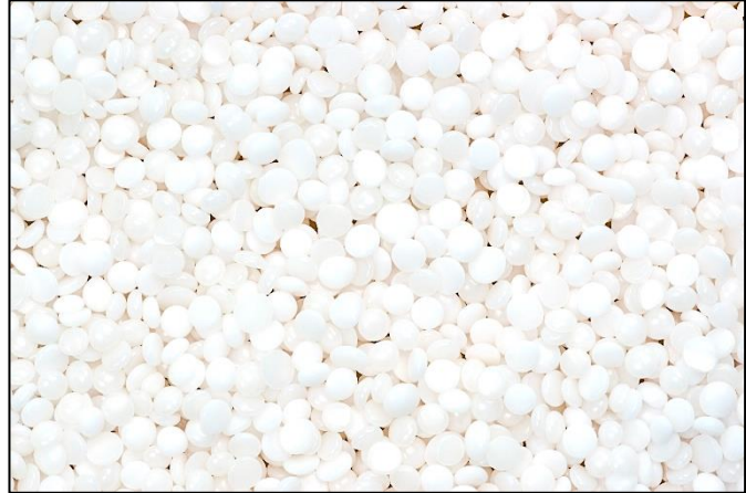
Figure 3, Feldspar granules with a highly reflective white ceramic coating for asphalt roofing shingles.
