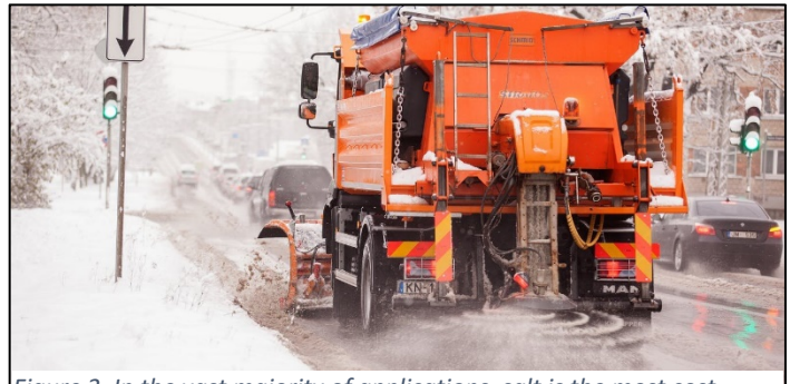
Figure 3. In the vast majority of applications, salt is the most cost-effective method for removal of ice from road surfaces.
